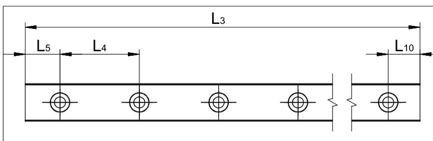
L<sub>3</sub> = standard rail lengths in mm
