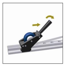
Tilt the tool forwards and move it along the rail so that the strip is pressed into its groove over the entire length of the rail.
