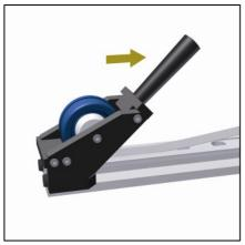
Turn the installation tool around and fit it to the rail again. The handle must point in the direction of installation.
