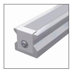
For more severe mechanical stress, e.g. when directly exposed to machining swarf, the strip ends can be secured with steel angles instead of the red plastic end pieces. In this case, the strip ends must be cut off at right-angles and free of burrs, and a thread for a mounting screw tapped in each end of the rail. Retro-fitting with steel strip retainers is therefore only recommended where induction-hardened rails are used.
