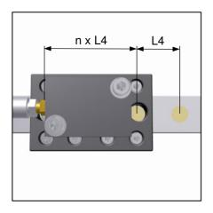
Slide the installation tool over the plug and position it centrally. The pressing position is reached when the two external inspection holes, or the cut-outs in the tool are over a rail mounting hole. Depending on the size, the inspection holes may be one or two pitches (L4) from the installation position. Please note:
