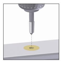
Use a suitable tap to cut a metric thread in the plug. Then clean any remaining swarf from the thread and hole.
