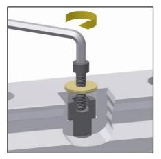
Turn the screw further with a suitable hexagon key. This action will draw the plug upwards out of the bore, see figure on the left. Continue to turn the screw until the plug has been extracted and can be removed by hand.
