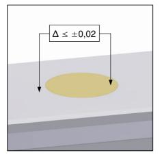
After pressing in all the plugs, check that they are correctly seated. The maximum permissible difference in height between the rail and surface of a plug is +/-0.02 mm measured at the edge of the plug. If necessary, repeat the pressing operation at a higher pressure until the correct position is reached.
