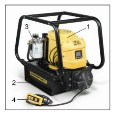
A normal, commercially-available hydraulic unit is required to supply pressure for the installation tool. As a rule, this consists of an electric motor driving a pump (1), an oil reservoir (2), a pressure regulator with a pressure gauge (3) and an operating panel (4).
