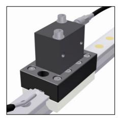
Blow compressed air through the gap between the sliding shoe and the upper surface of the rail to clear any swarf adhering to the punch.
