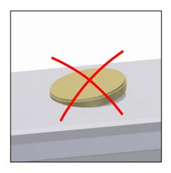
Ensure that the face of the plug is plane parallel to the upper surface of the rail.
