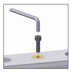
Screw a hexagon socket screw into the plug by hand until the end of the screw contacts the rail mounting screw.
