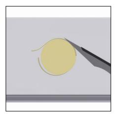
Operate the hydraulic cylinder for just a short period from the control panel until a click can be clearly heard. Then release the operating button immediately so that the cylinder returns to its original position. Push the installation tool to one side. The plug is now pre-installed and projects 0.2-0.3 mm above the upper surface of the rail.
