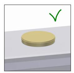
Place the plugs in the rail holes with the smaller end of their taper downwards.
