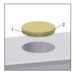
MRS brass plugs are tapered externally (1). The outside diameter is slightly larger than the bore diameter in the rail. During installation, material is displaced and sheared off; this is assisted by a stepped ring adjacent to the upper surface of the plug (2). This creates a gap-free, liquid-tight interference fit between the plug and the bore in the rail. This ensures, besides a secure fit for the plug, an optimum running surface for the carriage wipers.
