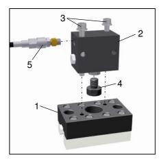
For correct installation of brass plugs, SCHNEEBERGER recommends the hydraulic installation tool MWH. This consists of a size-dependent MWH sliding shoe with punch and the universal hydraulic cylinder MZH; it must be ordered separately. The cylinder is a single-acting block cylinder with spring return.
