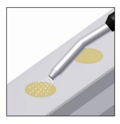
Use compressed air to blow the lose chip from the upper surface of the rail. If necessary remove any residual swarf with a brass brush. Check that all swarf has been removed completely.
