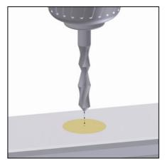
Make a centre-punch dot in the middle of the plug to be removed and drill carefully through the centre of the plug using an electric drill. Take care not to damage the rail mounting screw. The drill diameter should be the core diameter of the thread to be cut in the plug.
