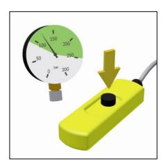
Switch on the hydraulic unit and set the desired pressure on the pressure regulator.
