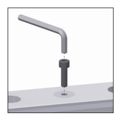
Screw a hexagon socket screw into the plug by hand until the end of the screw contacts the rail mounting screw.
