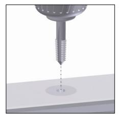
Use a suitable tap to cut a metric thread in the plug. Then clean any remaining swarf from the thread and hole.
