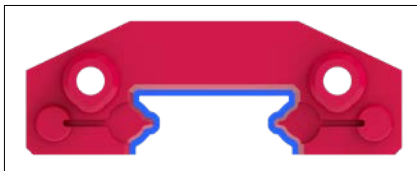
Standard wiper (blue contour = contact surface)
